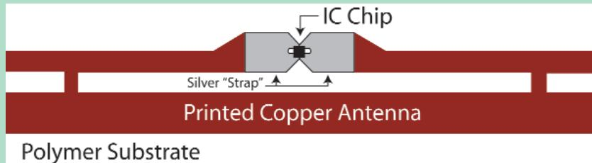
The modulated carrier wave transmitted by the interrogator is sensed by the antenna. The carrier wave induces a small alternating current (AC) in the antenna. Inside the IC chip, a power rectifier and regulator converts the AC to stable DC and uses it to power the IC chip, which immediately “wakes up.” The clock extractor separates the clock pulses from the carrier wave and uses the pulses to synchronize the logic, memory, and modulator sections of the tag’s IC chip with the interrogator.
