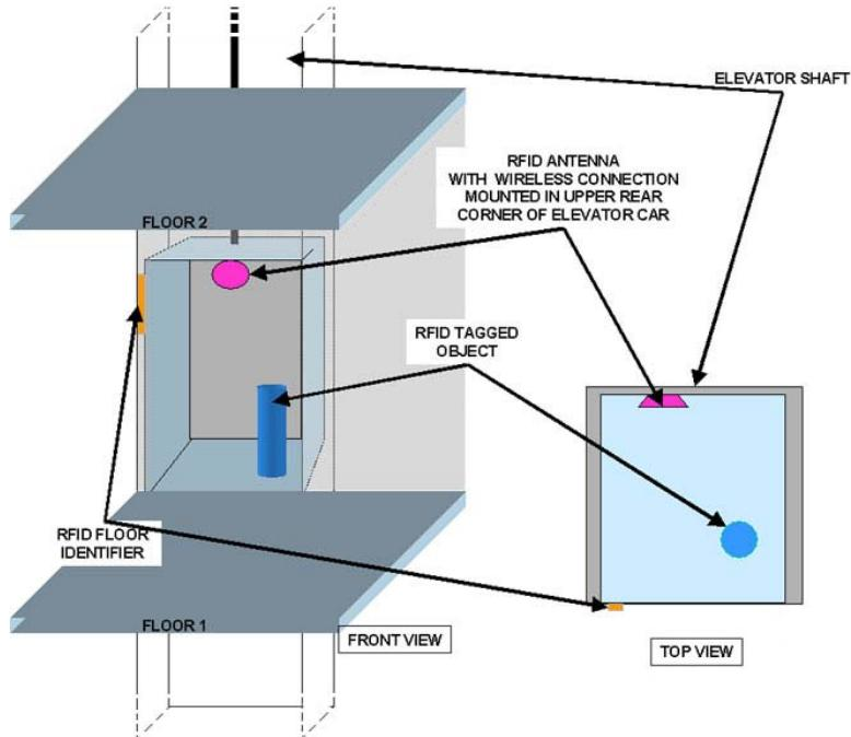
MVS has successfully tested this concept in elevators. The elevator system hardware is virtually identical to our forklift-mounted system currently in operation at Atlanta Data Storage in Norcross, GA ( Appendix C).
